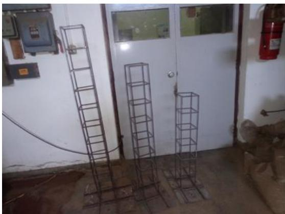
Figure 5: Sample of unbraced model structures
